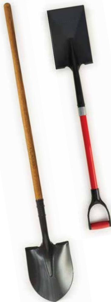
**SHOVELS** Gardeners should have at least two shovels: a round point for digging, a flat edge for edging. A long handle gives leverage, a D-handle aids lifting.
